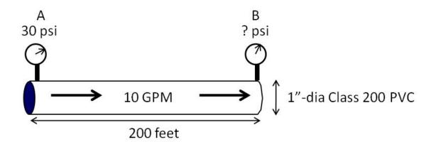
PVC CLASS 200 PIPE - Pressure Loss (psi/100 feet)
