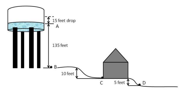
Water pressure at B: \_\_\_\_\_\_ feet of head, \_\_\_\_\_ ps
