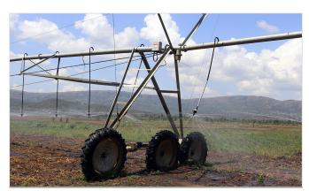
Figure 15. Wheels and pivot components catching and concentrating irrigation water at the towers/wheels.
