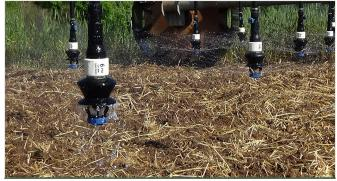
Figure 8. An example of a water applicator used for close drop spacing systems that can be easily switched to the bubble mode (LEPA) and spray mode (LESA).
