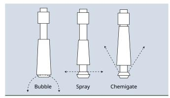
Figure 10. Original multi-functional LEPA head.
