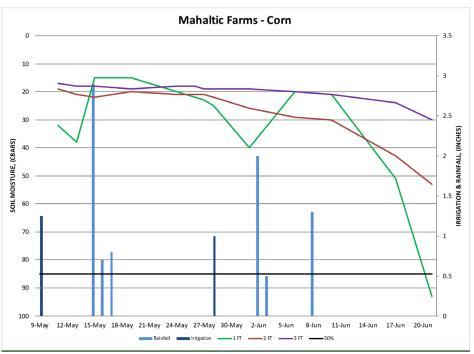
Figure 17. Soil moisture measurements in a corn field on a heavy clay soil. Soil moisture levels should not fall below a reading of 85 for this particular soil.
