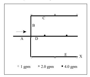
Complete the following table for the above system design. Choose the appropriate pipe diameter while limiting water velocity to 5 ft/sec. Use the friction loss chart provided for **Class 200 PVC** pipe.
