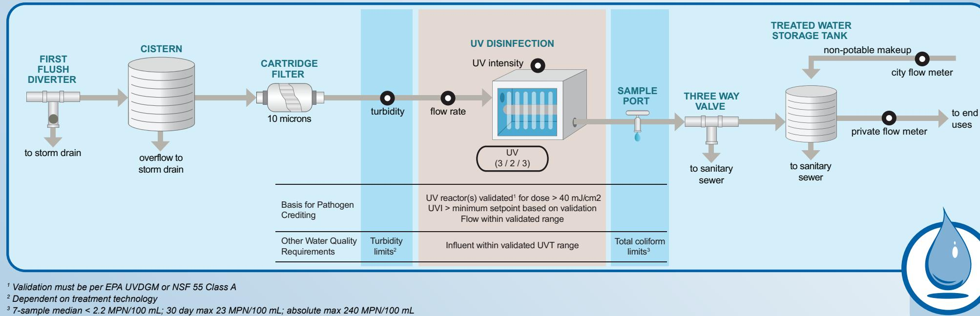
For rainwater, the only specified LRT is for protozoa. In this example, the LRTs are met with a validated UV reactor that operates within certain operating conditions. The inclusion of a cartridge filter upstream of the UV reactor provides pre-treatment to improve the water quality of the water prior to disinfection and helps meet the turbidity limits. Because the use is outdoors, no chlorine residual is required.
